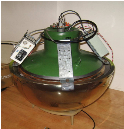
Quasar-370 D \approx 14.6'' Quantum efficiency \approx 0.15
