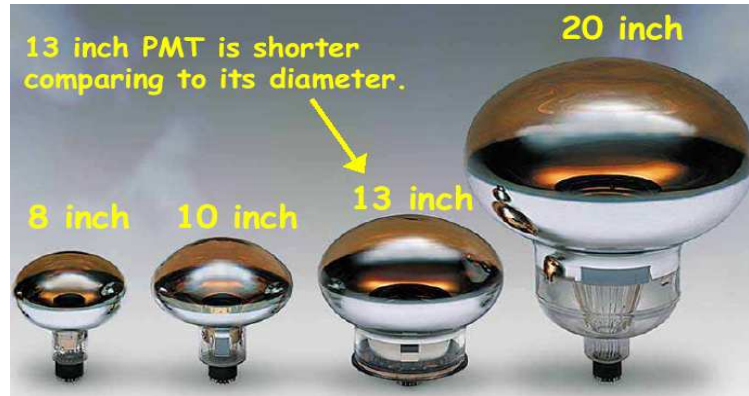
Hamamatsu R8055 D \approx 13'' Quantum efficiency \approx 0.20
