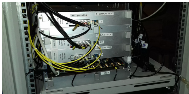
Figure 6: The 4-Channel TDC in application: nsec-monitoring of the TAIGA central timing system (GPS, GPSDO, WRS-Master and -network) by three 4-channel SPEC TDCs and a ZEN TDC.
