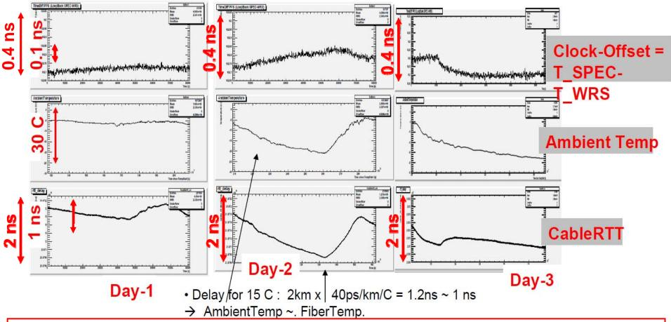
The fiber delay, induced by ambient temperature variation, are compensated by WR to < 0.2 ns level
