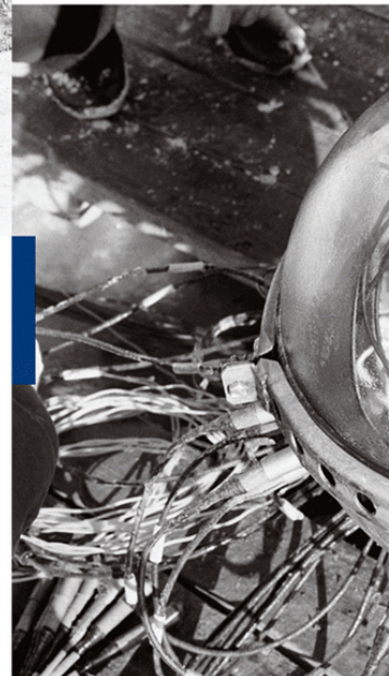
Above: A frigid, rustic campsite is home to the scientists who maintain the Baikal Neutrino Telescope. Right: One of the telescope's 228 detectors, which pick up flashes of light triggered by passing neutrinos.
